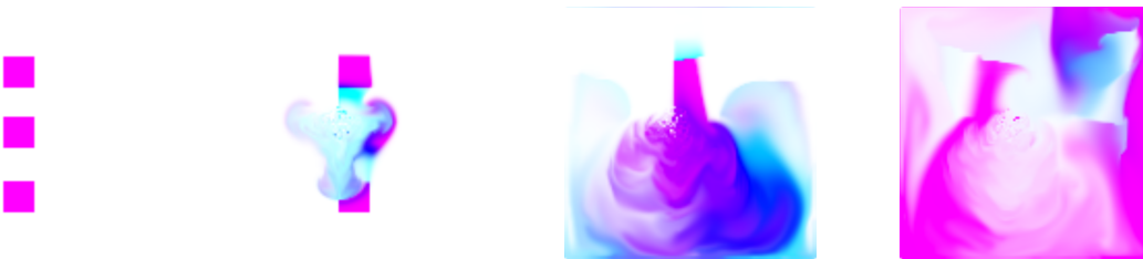
Figure 4. The constant velocity source is at the upper left corner of the central square in the initial conditions (leftmost image). Initial conditions also had dye in layers below the uppermost layer, though only the uppermost layer is rendered. This leads to evolution over time of the color of the fluid exiting the constant velocity source, as dye is transported underneath the surface and eventually pulled up by the constant velocity source or by other convection cells. Note the sharp edges visible in the rightmost image. These appear to be fluid separations from vertically-oriented convection cells, and are extremely unrealistic; during the simulation, these separations persist for quite a while. If fluid is flowing under the topmost layer, blending the top few layers of the fluid may solve this problem while also better approximating the appearance of milk. Note also the excessive diffusion of dye, despite a null diffusion constant; this is a consequence of numerical dissipation as discussed previously.
